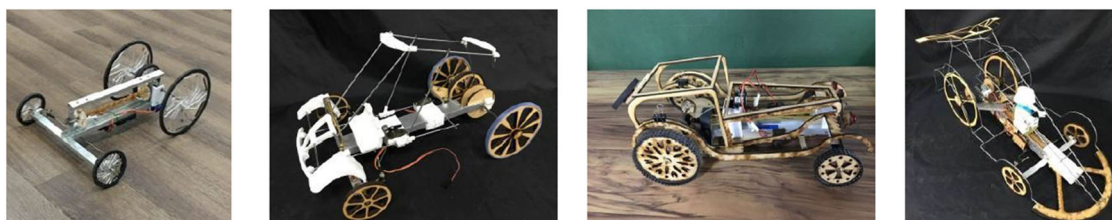
Fig. 3 Teachers' coursework. Technology teachers used STEM knowledge and steering and torque release strategies to design various elastic cars.
