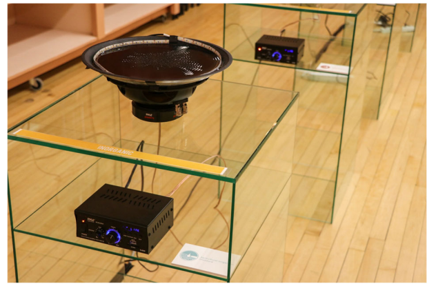
Fig. 3 Ripple Effect details. Each sound station includes: One speaker, one amplifier, a bowl filled with water, a strip of LED lights attached to the rim of the bowl, an Arduino, a label stating the contaminant, and a label stating the comparative value. Installed at the Bullion Plaza and Cultural Museum, Globe, AZ, USA. Reproduced from Kaufmann et al. (2021).
