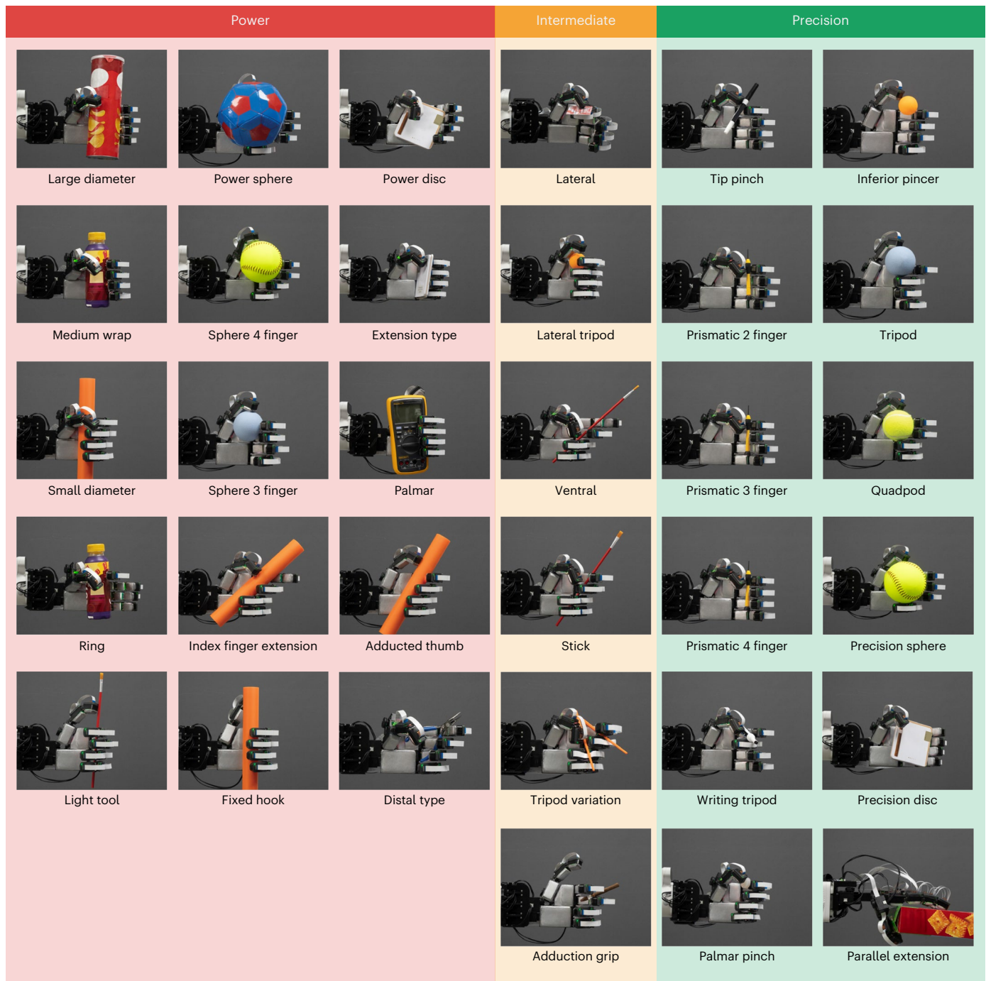
Fig. 3 | Workspace of F-TAC Hand. Empowered by its smart design, the workspace of F-TAC Hand enables it to perform all 33 human grasping types, as documented in ref. 24.
