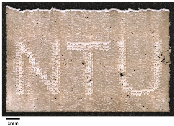
Fig. 2 | Cross-sectional optical micrograph of an architected sample containing un-tempered \alpha' -martensite (white) consolidated in a configuration which produces the acronym “NTU”.
