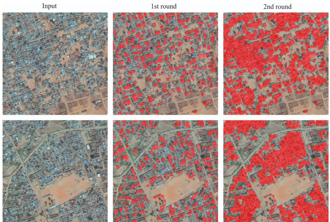
Figure 2. Building map improvement following two rounds of training. The network learns to group dense buildings when trained with small amounts of additional data that are similarly labeled. Extracted buildings are marked in transparent red.
