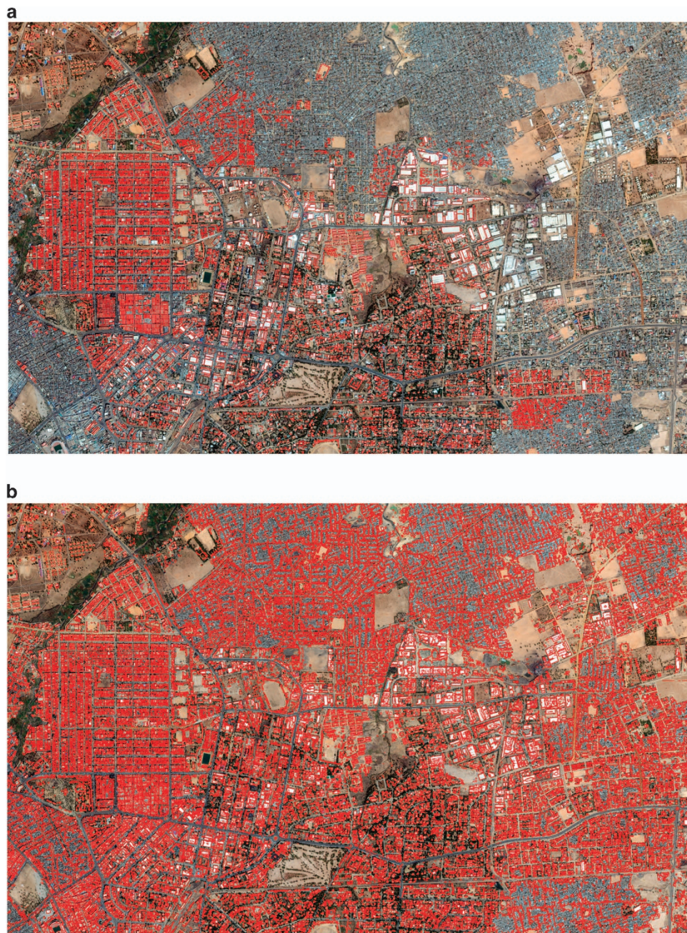
Figure 4. Comparison of map completeness for Kano city. (a) Building map generated using OSM data. (b) Building map generated using our approach. Building boundaries are marked in red.
