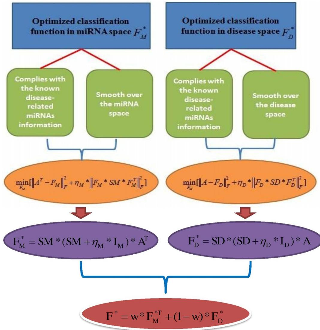
**Figure 3** | The flowchart of RLSDMA includes three steps: solving optimization problem; obtaining the optimal classifier in the disease and miRNA space, respectively; combining classifiers in the disease and miRNA space to obtain final predictive result.
