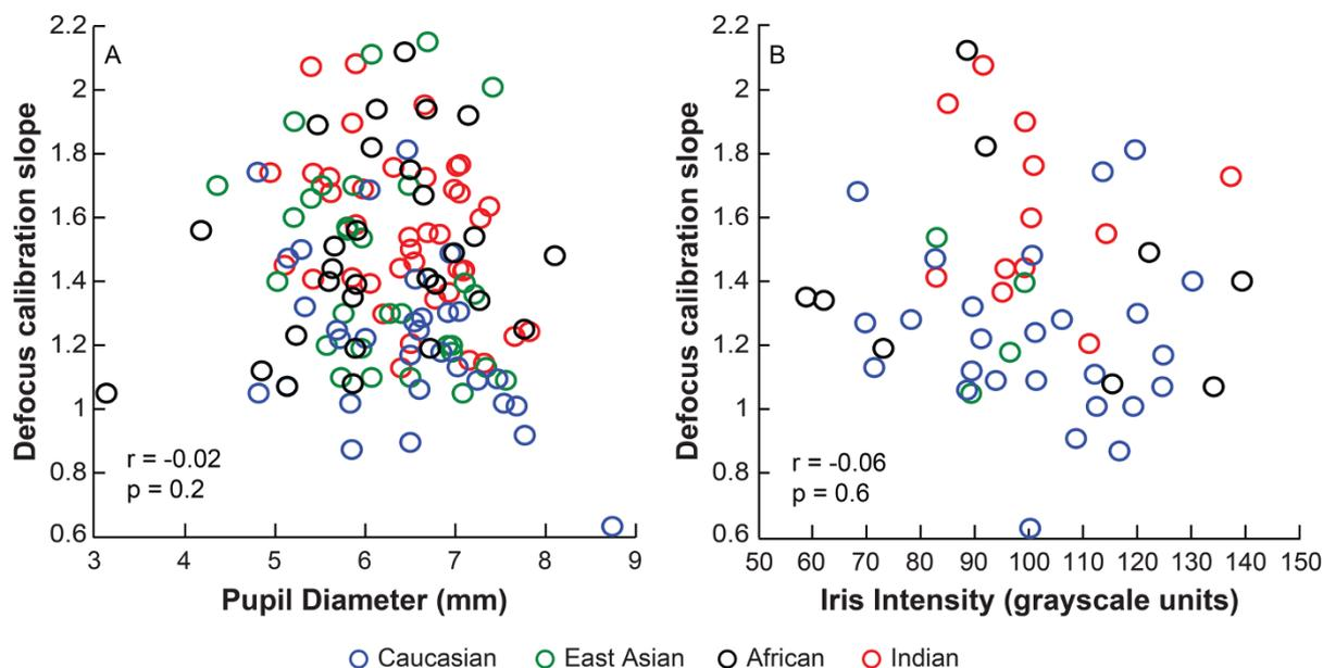
**Figure 4** | Scatter plot of the defocus calibration factor of each subject plotted against their respective pupil diameter (panel A) and grayscale iris intensity (panel B). Data from different ethnic groups are indicated in different colors.
