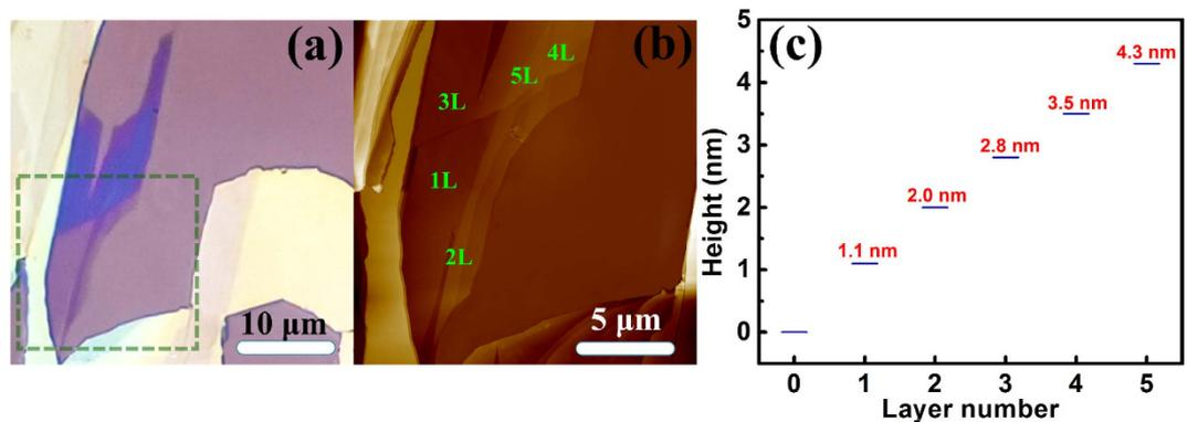
**Figure 3. Microscopic Imaging.** (a) Optical microscopic images of mono- to multilayer WTe<sub>2</sub> on a Si substrate with a 300 nm SiO<sub>2</sub> layer. (b) AFM image of the area (20 × 20 μm<sup>2</sup>) surrounded by a green dashed line in (a). (c) Height of the flake as a function of the layer number.
