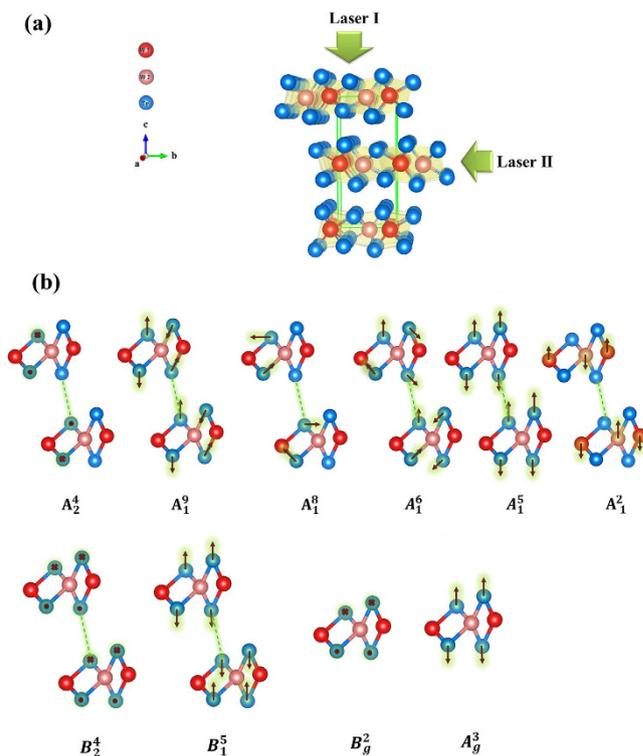
**Figure 1. Lattice structure.** (a) Crystal structure of  $\text{WTe}_2$  along the  $a$ -axis direction, showing the orthorhombic unit cell. (b) Atomic displacements of Raman active modes in  $\text{WTe}_2$  bulk and monolayer. Here, “ $\times$ ” and “ $\circ$ ” indicate that the Te atoms move into and out of the  $bc$  plane, respectively.
