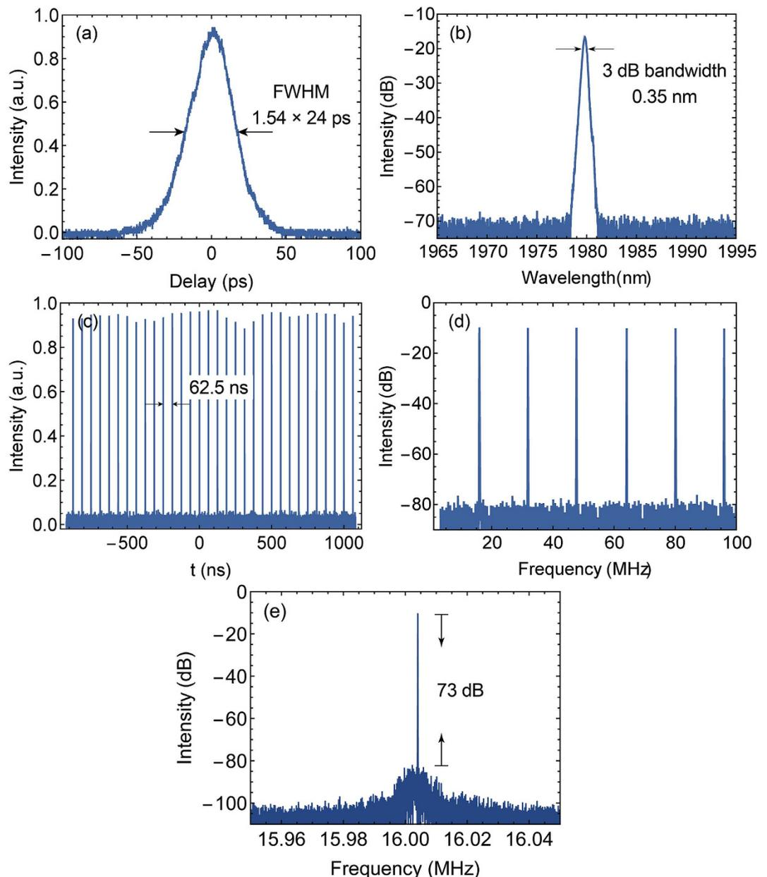
**Figure 2.** (a) The autocorrelator trace; (b) The optical spectrum; (c) The oscilloscope trace; (d) The RF spectrum of the output pulse under the pump power of 220 mW; (e) The RF spectrum with the span of 100 kHz and resolution bandwidth of 10 Hz.
