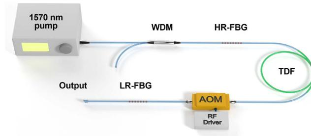
**Figure 1.** The schematic diagram of the FBG-pair-based FSF mode-locked fibre laser. TDF, thulium-doped fibre; WDM, wavelength division multiplexer; HR-FBG, high-reflectivity fibre Bragg grating; LR-FBG, low-reflectivity fibre Bragg grating; AOM, acousto-optical modulator; RF driver, radio frequency driver.
