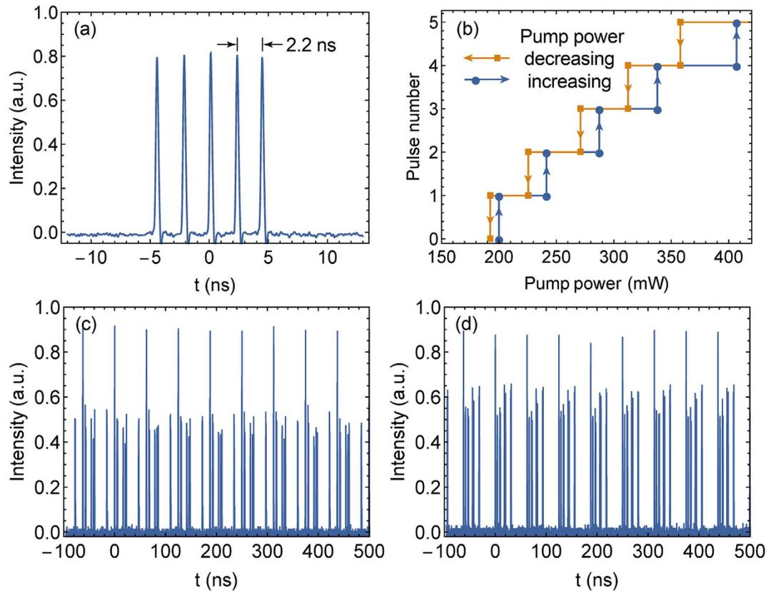
**Figure 3.** (a) The oscilloscope trace of the 5-pulse-bundle; (b) The variation of the number of the sub-pulses versus the increasing and decreasing pump power; The oscilloscope trace of the output pulse train under the pump power of (c) 0.6 W and (d) 0.9 W.
