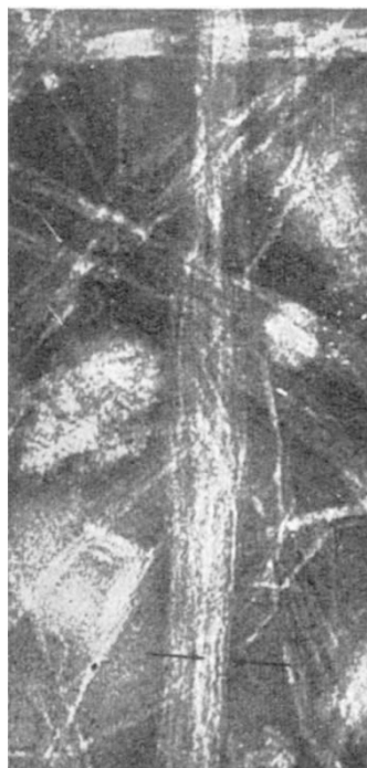
Fig. 1. Merino wool reduced, dispersed by ultrasonic irradiation, and stained with phosphotungstic acid ( \times 275,000 )
