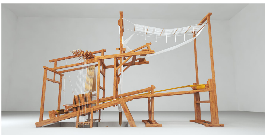
Fig. 8 | Restoration effect drawing (Side view) of the Yunjin Dahualou Loom.
