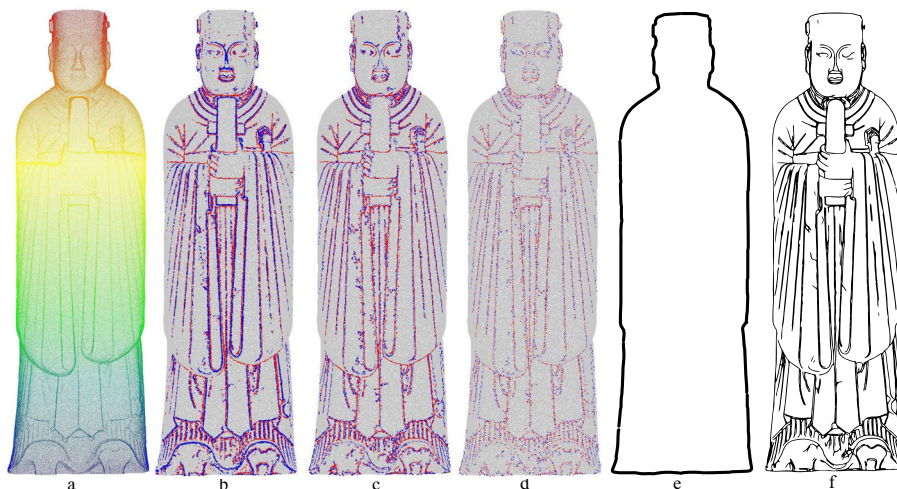
Fig. 6 | Overall process. a Input point cloud. b Feature points, with red indicating ridge points and blue indicating valley points. c Refined feature points. d Sparse points. e Boundary points. f Archeological line drawings.
