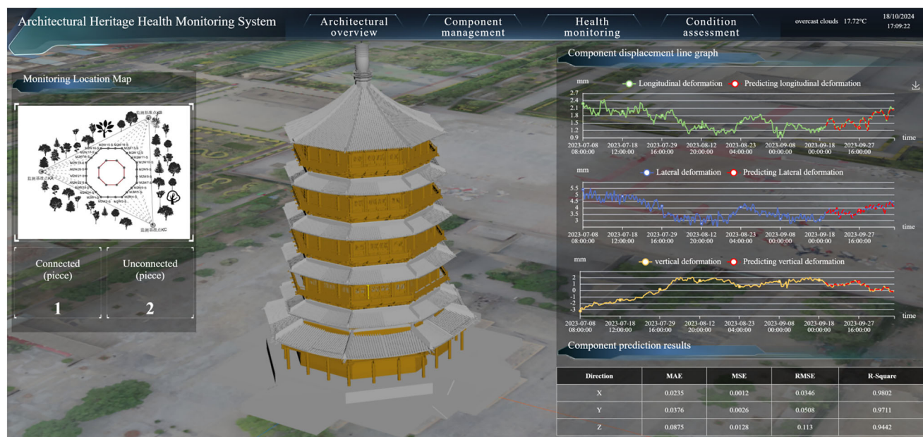
Fig. 8 | Digital twin behavioral model visualization system.
