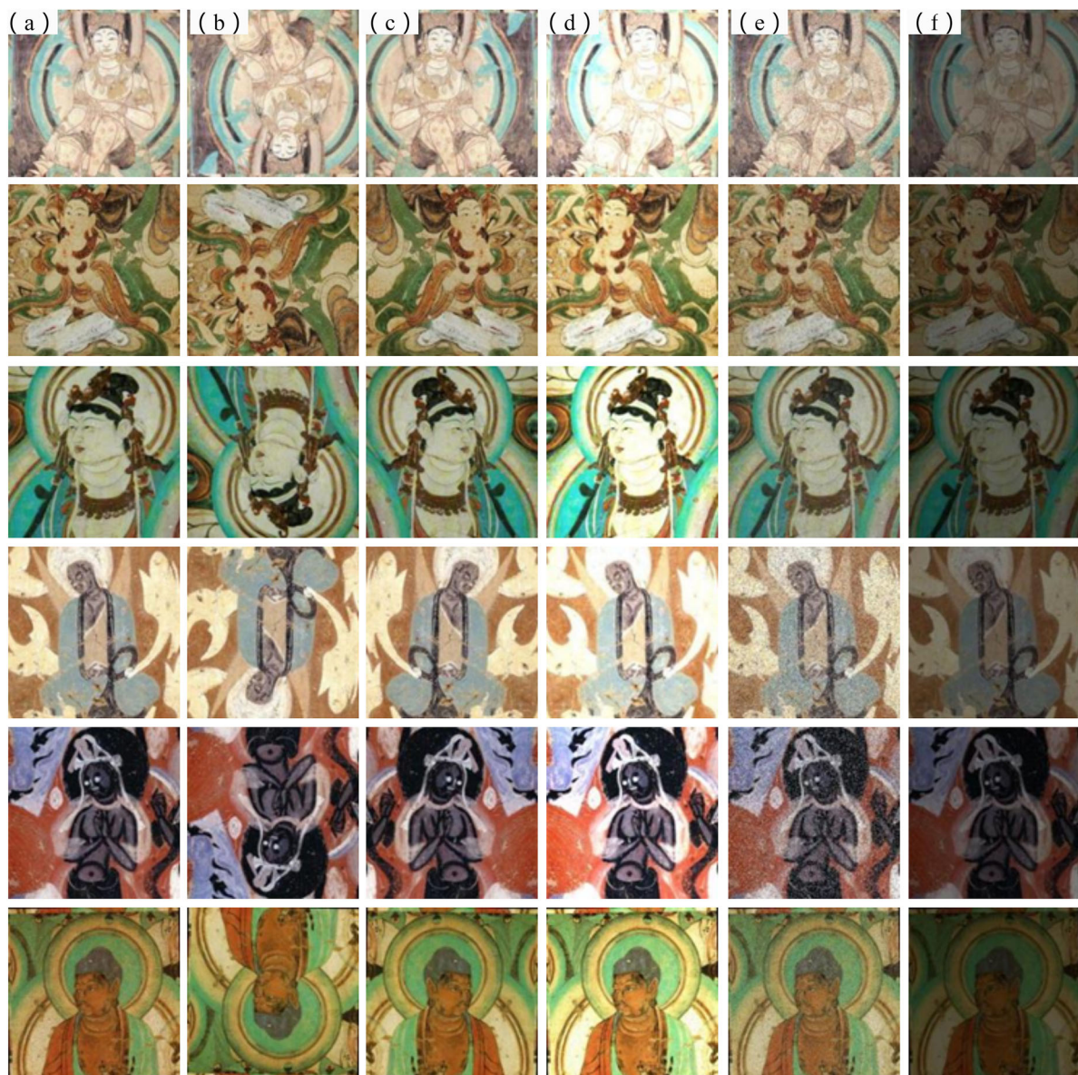
Fig. 7 | Schematic diagram of image data enhancement for each dynasty. (a) Scaling (b) Vertical Flip (c) Horizontal Flip (d) Increase Brightness (e) Salt-and-Pepper Noise (f) Decrease Brightness.
