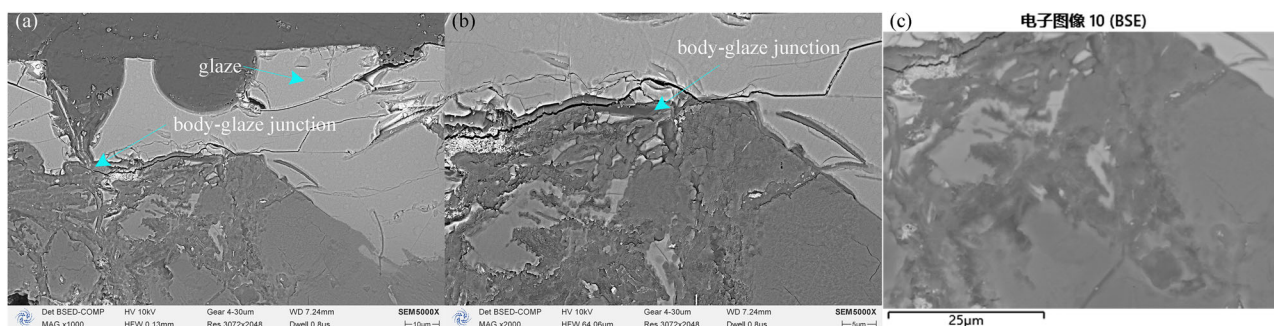
Fig. 4 | Scanning electron microscope images of the glaze-body join in sample YYQL061. a SEM image of the glaze-body join in sample YYQL061 at 1000× magnification, showing the bonding relationship between the glaze and body. b SEM
