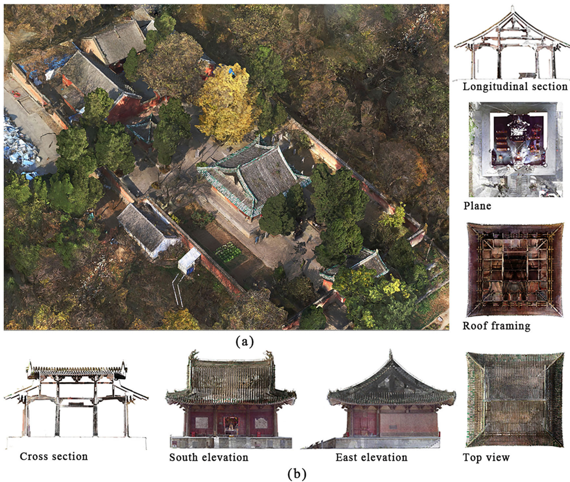
Fig. 14 | 3D reality model and point cloud slice drawing. a 3D reality model. b Point cloud slice drawing. It includes longitudinal section, plane, roof framing, top view, east elevation, south elevation and cross section.
