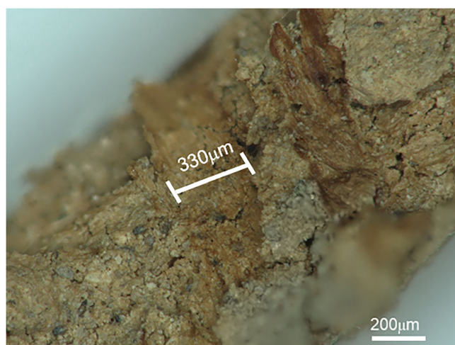
Fig. 10 | Image of the side of a single strip-shaped core with marks caused by the fabric layer under extended depth-of-field microscopy. scale bar: as indicated; ruler tick: marks denote distance ( \mu\text{m} ).
