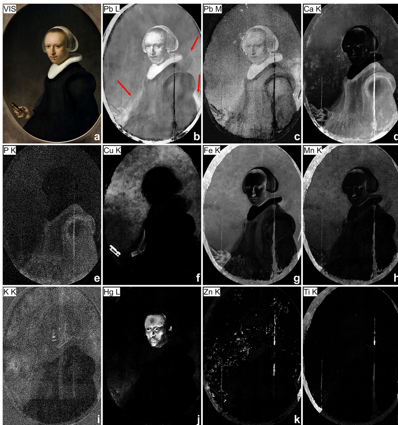
Fig. 2 | Portrait of a 39-Year-Old Woman. Elemental distribution maps obtained by XRF mapping: Pb La (b), Pb M (c), Ca K (d), P K (e), Cu K (f), Fe K (g), Mn K (h), K K (i), Hg L (j), Zn K (k), and Ti K (l). In b, the arrows indicate adjustments that
