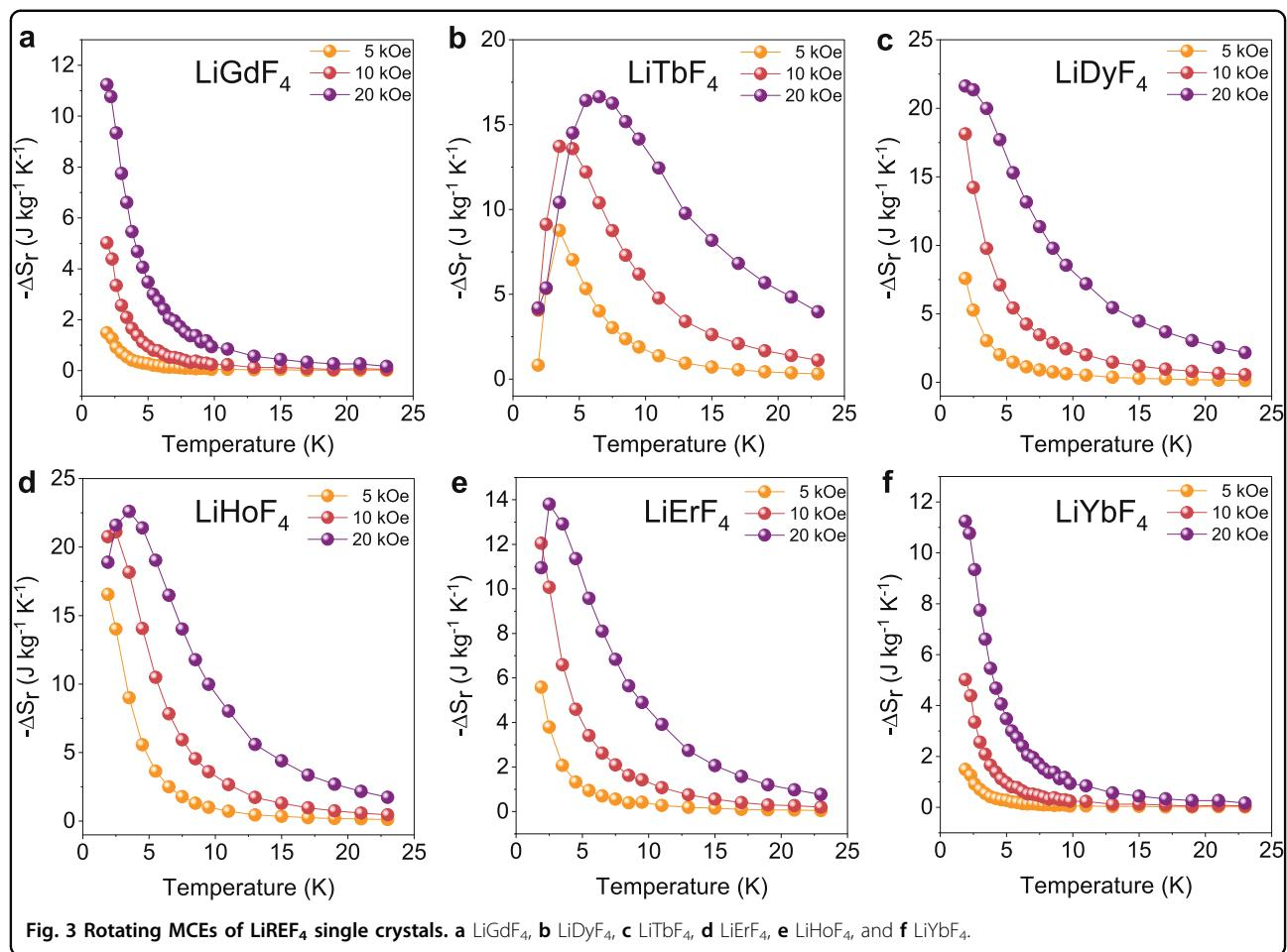
**Fig. 3** Rotating MCEs of  $\text{LiREF}_4$  single crystals. **a**  $\text{LiGdF}_4$ , **b**  $\text{LiTbF}_4$ , **c**  $\text{LiDyF}_4$ , **d**  $\text{LiErF}_4$ , **e**  $\text{LiHoF}_4$ , and **f**  $\text{LiYbF}_4$ .
