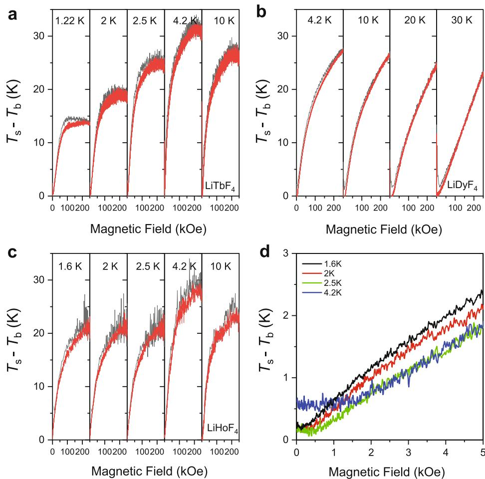
**Fig. 4 Adiabatic temperature changes of  $\text{LiREF}_4$ .** The temperature change  $T_s - T_b$  of  $\text{LiTbF}_4$  (a),  $\text{LiHoF}_4$  (b), and  $\text{LiDyF}_4$  (c) measured with pulsed magnetic fields applied along easy axes. d The temperature change  $T_s - T_b$  of  $\text{LiHoF}_4$  when magnetic fields ramped from 5 kOe down to 0.
