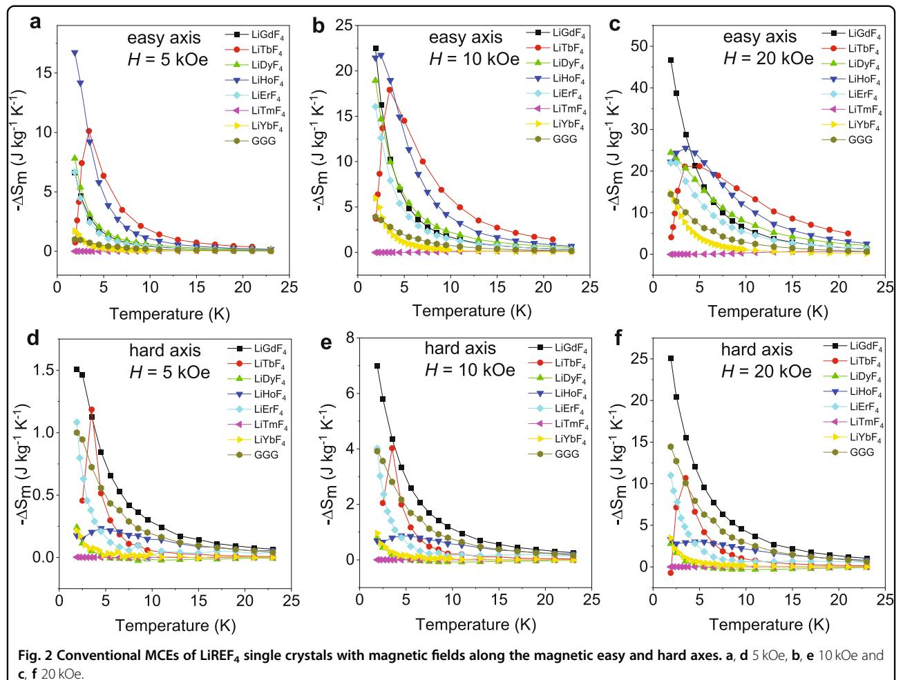
**Fig. 2** Conventional MCEs of  $\text{LiREF}_4$  single crystals with magnetic fields along the magnetic easy and hard axes. **a, d** 5 kOe, **b, e** 10 kOe and **c, f** 20 kOe.
