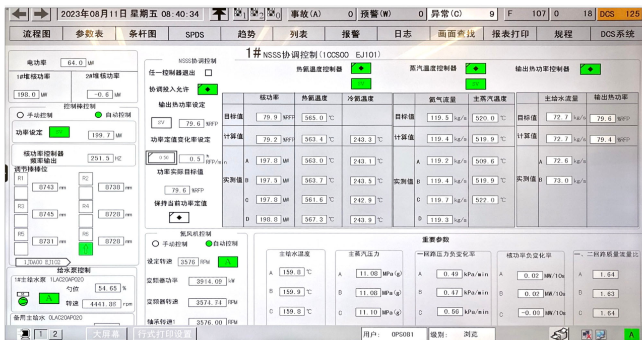
Fig. 5 | Human machine interface (HMI) of the coordinated control system. This HMI is running on the operator station of #1 module.
