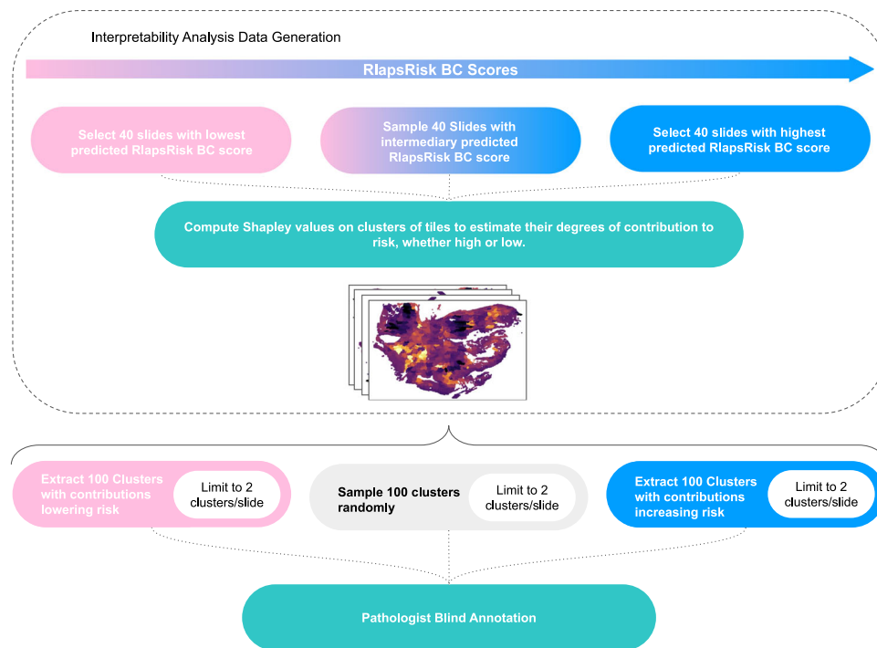
Fig. 5 | Interpretability of the RlapsRisk BC model. The methodology applied to generate the data used for this analysis is outlined. To streamline pathologist review, slides were sampled to express as much diversity as possible in the high, low, and intermediary predicted risks. Shapley values were computed to evaluate
