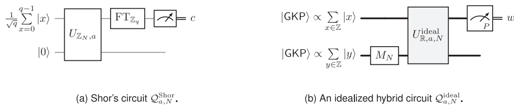
Fig. 4 | Contrasting Shor's circuit with an idealized hybrid circuit Q_{a,N}^{\text{ideal}} . Instead of modular exponentiation followed by Fourier transform and computational-basis measurement in Shor's circuit (a), our idealized hybrid circuit Q_{a,N}^{\text{ideal}} (b) employs
