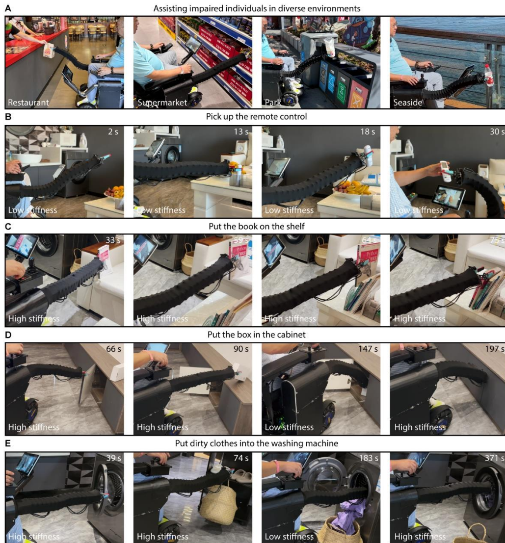
Fig. 6. Validation of the BRT-assisted wheelchair in real-world scenarios by a post-stroke individual. (A) The BRT-assisted electric wheelchair supports daily activities across diverse real-life environments, including a restaurant, supermarket, park, and seaside. (B) Task: Pick up the remote control. The BRT operates in a low-stiffness mode to enable compliant reaching and gentle grasping of lightweight objects. (C) Task: Put the book on the shelf. The robot maintains a high-stiffness state to support the weight of the book and ensure precise placement on an elevated shelf. (D) Task: Put the box in the cabinet. The BRT dynamically modulates between high and low stiffness to navigate confined space and execute stable placement. (E) Task: Put dirty clothes into the washing machine. The system adjusts stiffness in real time to facilitate both flexible positioning and robust object transfer, adapting to changes in posture and load.
