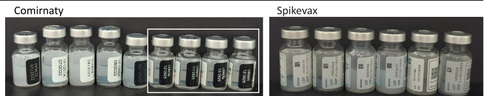
Fig. 10 | Photographs of vials containing analysed batches of Comirnaty and Spikevax vaccines. Non-expired vaccines appeared clear, while expired vaccines were visibly turbid. Batches within the expiration date are highlighted with a white rectangle.
