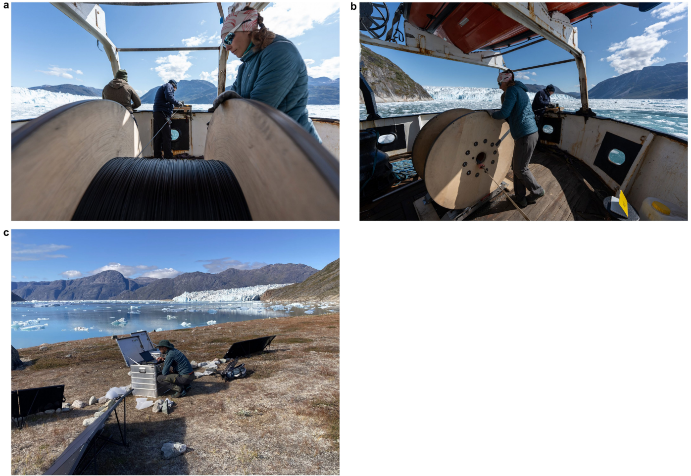
Extended Data Fig. 1 | Pictures of the fibre-optic cable deployment and interrogator setup. a/b, Pictures showing the manual deployment of the subsea fibre-optic cable from the ice ship R/V Adolf Jensen. a, View over the cable drum towards the cable counter and the stern of the vessel. b, Wooden cable drum was hand-propelled and controlled by one person. A second person supervised the cable length counting and synchronization of the deployment
