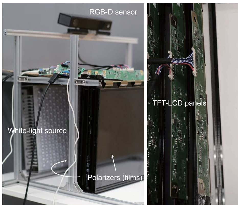
Extended Data Fig. 7 | The physical device of autostereoscopic display prototype. The white-light source is an LED array enclosed within the device, and orthogonal polarizer films are applied to on the front of the top screen and the back of the bottom screen in the LCD-panel stack.
