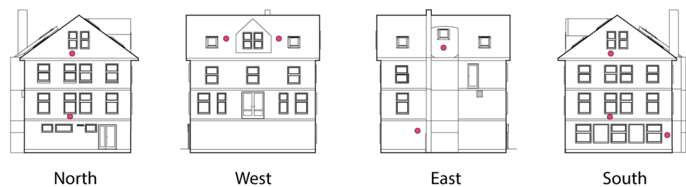
Fig. 5 Locations of the building façade temperature sensors.
