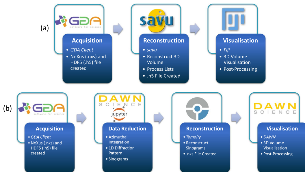
Fig. 4 Data processing pipelines for both (a) XCT data and (b) XRD-CT data from acquisition through to reconstruction to post-processing. Software and file formats are also indicated.
