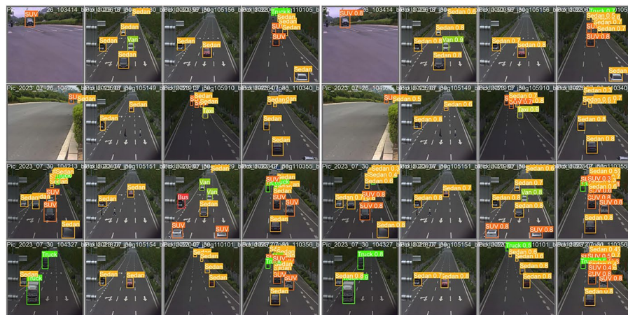
(a) Ground truth annotations and YOLO-predicted outputs of VIS model
