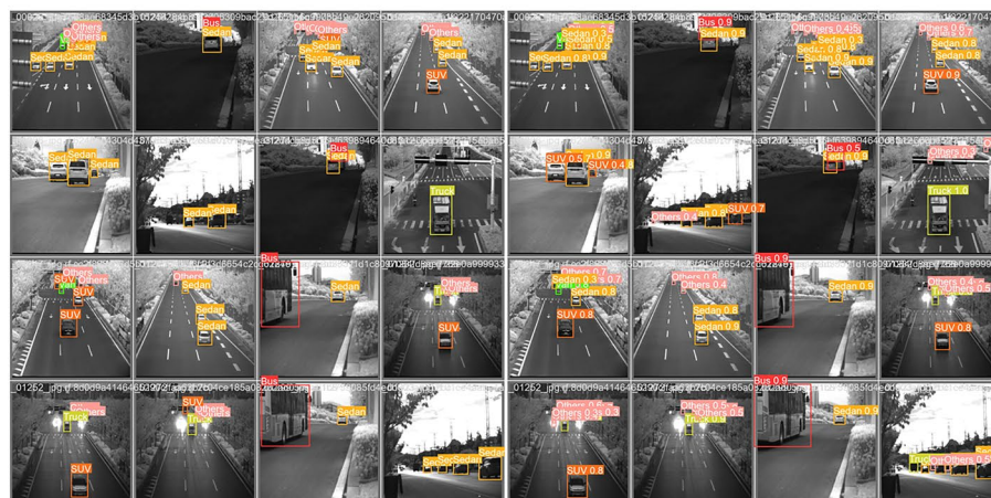
(b) Ground truth annotations and YOLO-predicted outputs of SWIR model
