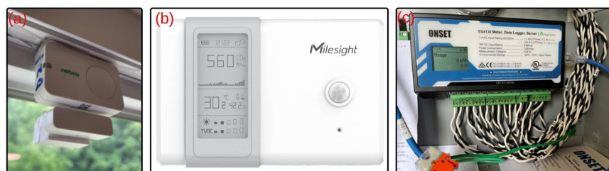
Fig. 4 This figure shows the three types of sensors used to measure window state, IEQ, and energy consumption by power circuit channels. (a) depicts window/door state sensors, while (b,c) show IEQ and power meter sensors, respectively.
