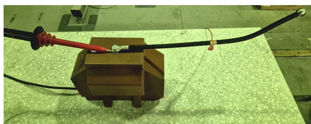
Fig. 15 Partial-discharge ( PD-only ) defect: epoxy block with an internal void connected to the same conductor.
