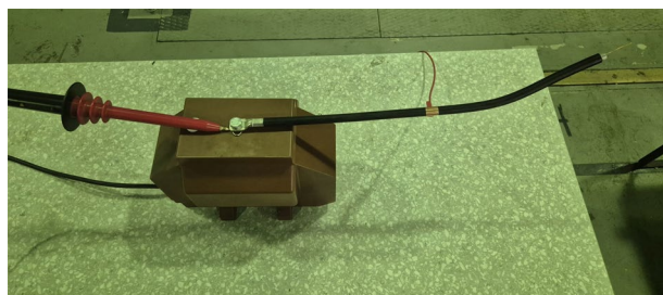
Fig. 14 Artificial corona-only defect: a sharpened needle connected to the energized conductor (12.7 kV) produces surface-corona discharges in air.
