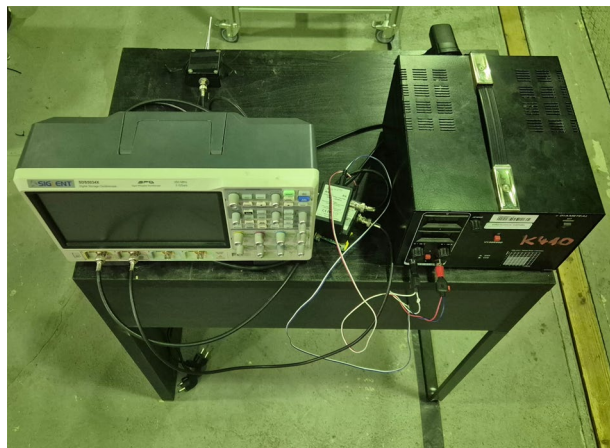
Fig. 13 Top-down view of the measurement chain, highlighting the RF front-end, coaxial cabling, and supply wiring.
