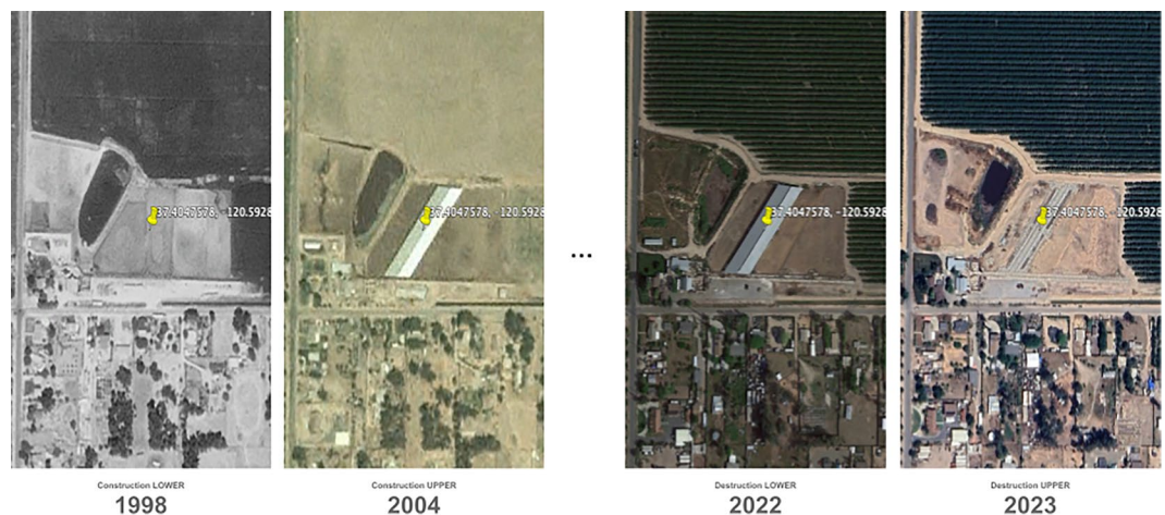
Fig. 4 An example of construction dating for a facility in California, showing the relationship between animal presence in satellite imagery and construction lower/upper and destruction lower/upper bounds in the dataset. The left panels depict the construction of a facility between 1998–2004 and the right panels depict the destruction of a facility between 2022–2023.
