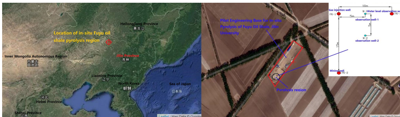
Figure 1. Location of oil shale in-situ pyrolysis region and layout of wells.
