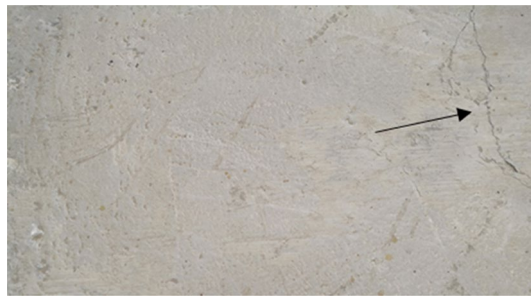
Figure 8. Diagonal cracks in a smooth specimen.
