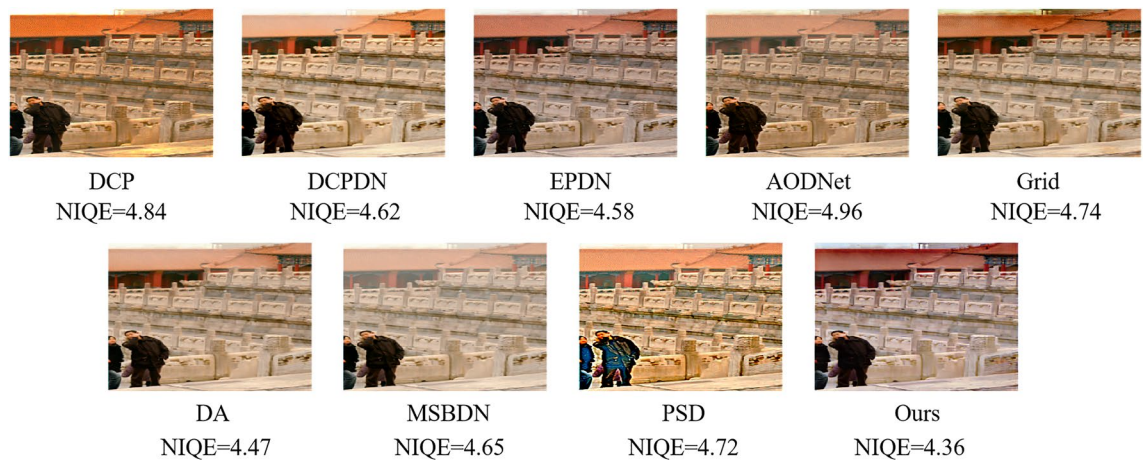
Figure 1. Comparative results on a real-world image using DCP, DCPDN, EPDN, AODNet, Grid, DA, MSBDN, PSD, and the proposed method. Natural Image Quality Evaluator (NIQE) is a non-reference criterion that is widely used in image quality assessment. Lower values of NIQE represent better performance.
