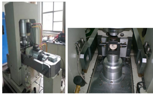
Figure 3. RMT-150B electrohydraulic servo rock test system.
