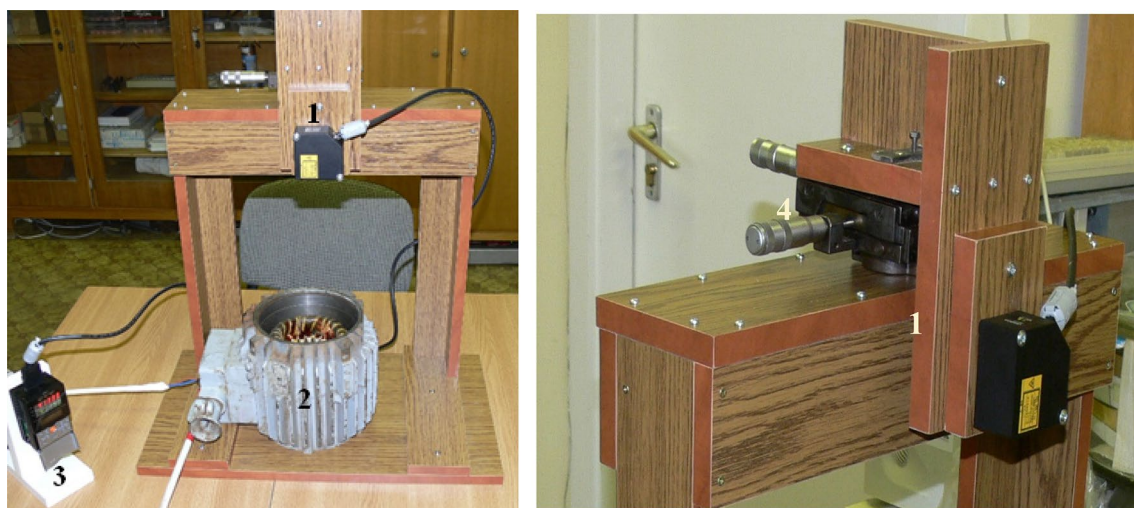
Figure 2. The unit for measuring the decrease in the level of the rotating metallic melt 1: laser, 2: inductor, and 3: display, 4: X - Y table.
