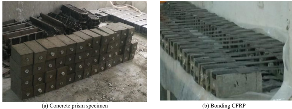
Figure 1. Fabrication of CFRP-concrete double shear specimens.
