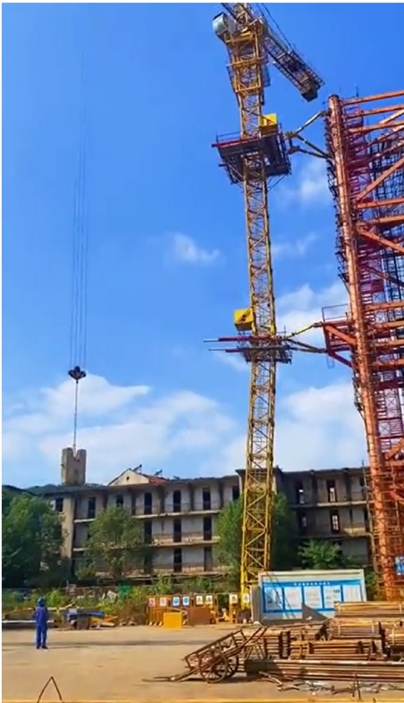
Figure 20. Hoisting test of the inclined tower crane.
