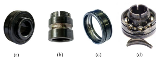
Figure 5. Normal and fault state of bearings (a) normal (b) inner race fault (c) outer race fault (d) ball fault.
