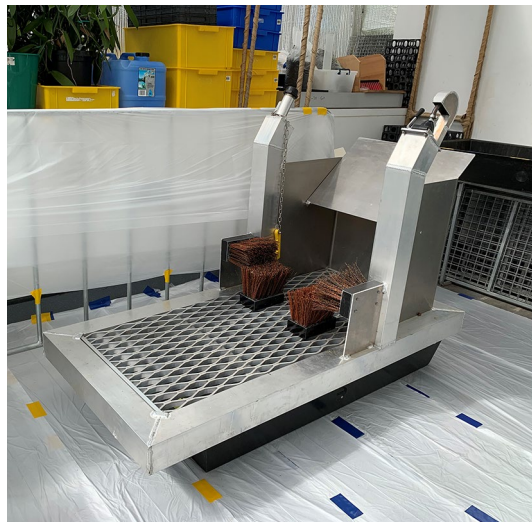
Figure 6. Hygiene station used in the study. The whole machine was placed on top of a large sturdy tub to catch soil particles through the grate. Note the fixed boot brushes, and the disinfectant spray lever on the right.
