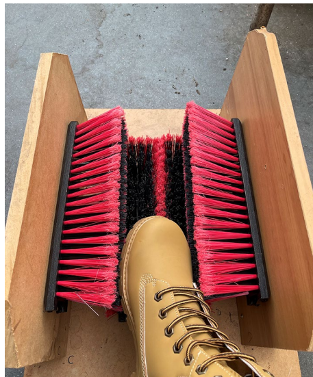
Figure 3. Fixed boot brush device, constructed from broom heads bolted onto timber sheets, used in the study.
