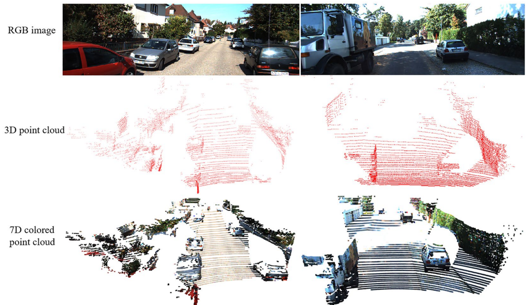
Figure 3. Some visual examples of RGB image, 3D point cloud and corresponding 7D colored point cloud.
