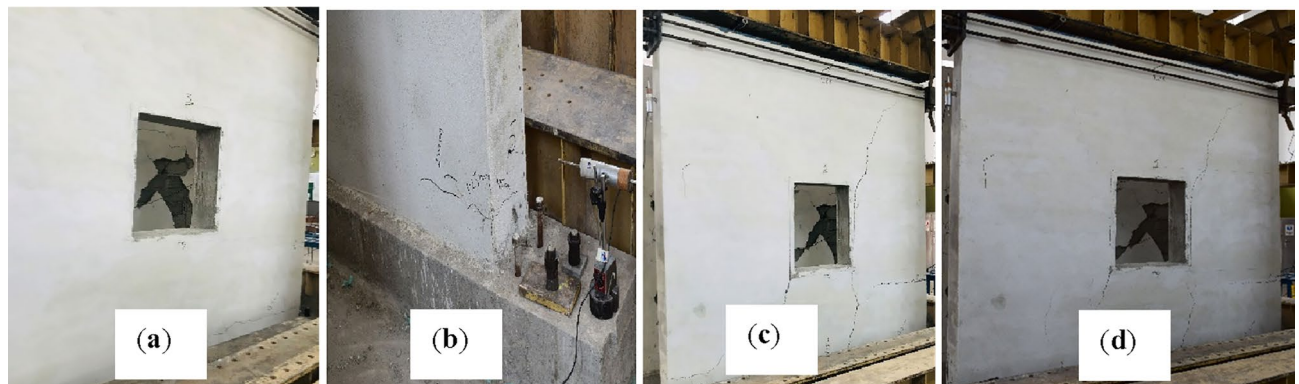
Figure 8. Damaged state of URM wall at storey drift ratios of (a) 0.04, (b) 0.06, (c) 0.52 and (d) 0.60.
