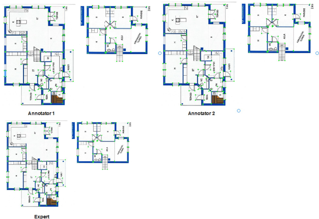
Figure 8. The first annotator missed 1 door and 2 windows, the second annotator 2 missed 1 window, the last one annotated by the expert.
