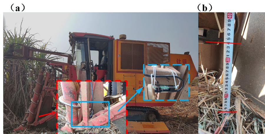
Figure 5. Field test situation map: (a) Distance measurement module installation location; (b) Actual height of the installation position from the ground 34 cm and vegetation cover thickness of sugarcane field 5 cm.
