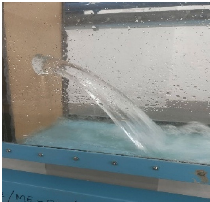
Figure 2. Plunging water jet with J_n = 1 .
