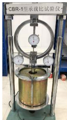
Figure 3. CBR-1 bearing ratio tester.
