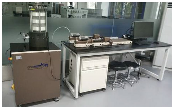
Figure 2. Dynamic triaxial test system.
