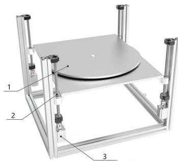
1. Rotating platform; 2. Lead screw module; 3. Stepper motor
