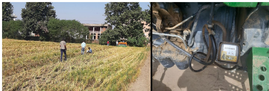
Figure 1. Test run of PSS to measure operational parameters like speed, slip and fuel consumption.
