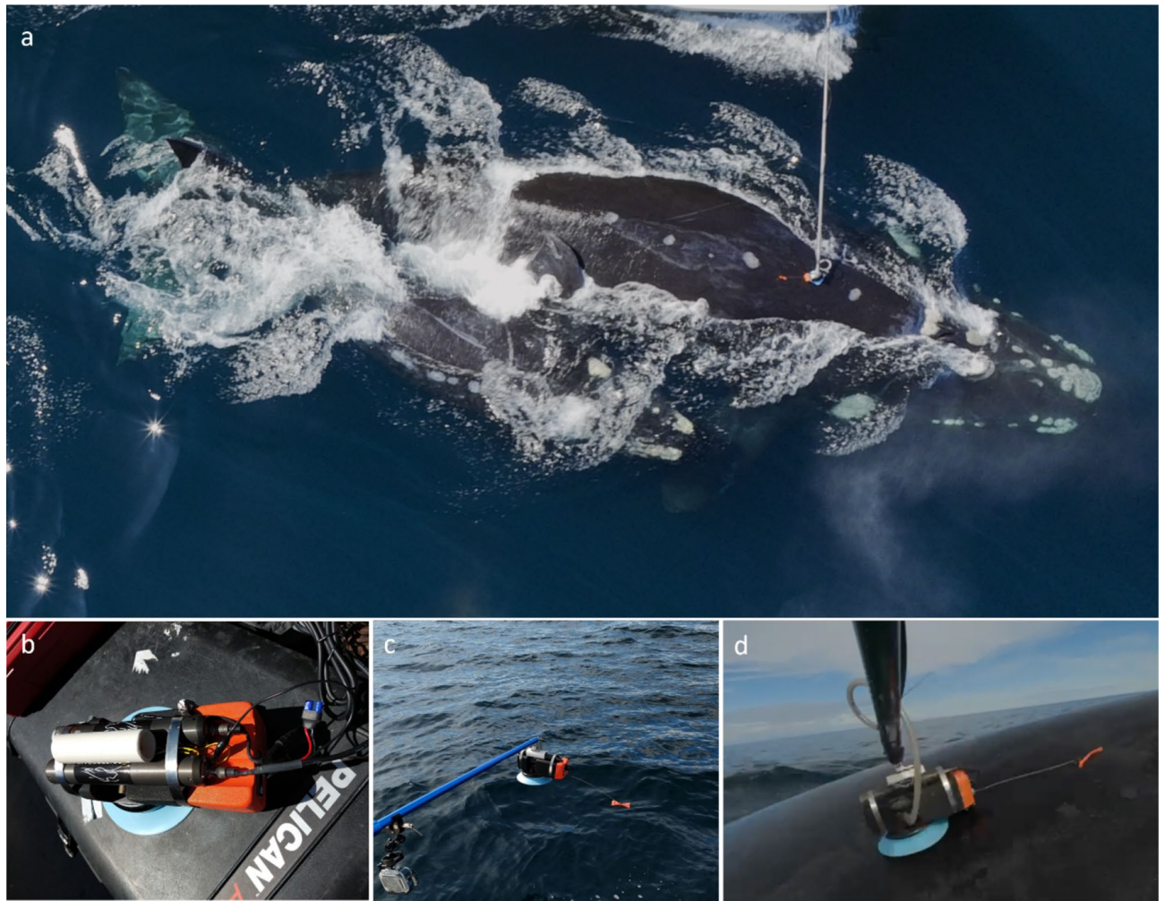
Figure 2. (a) CRITTERCAM deployments on southern right whales ( Eubalaena australis ) in Golfo Nuevo, (b) CRITTERCAM system, (c) CRITTERCAM system attached to deployment pole, (d) CRITTERCAM deployed on an individual southern right whale.
